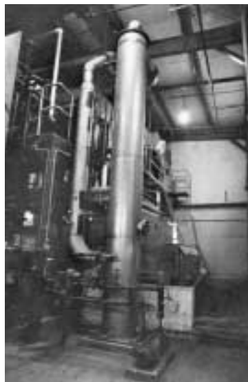
This unit efficiently recovers isopropyl alcohol from FMC's seaweed extraction process while reducing pollutants. The need for additional pollution instrumentation can be eliminated upon installation of units such as this one.
